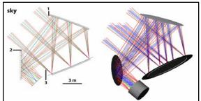
A possible optical layout of a crossed-Dragone telescope. Light from the sky is reflected first off a primary mirror, then off a similarly-sized secondary, and finally off a smaller tertiary. The combination permits a high throughput of the light over a very wide field of view and delivers a flat focal plane that can accommodate hundreds of thousands to millions of detectors. From Niemack (2016, Appl. Optics, 55, pp. 1688-1696; arXiv:1511.04506).
